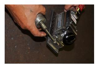
Step # 4 With pad removed, oil the right and left runner assemblies. Again be generous with the lubricant.
