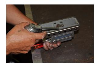
Step # 5 Lastly squirt a generous amount of oil in the center pad mounting screw hole. It's best to let the tool sit a few hours or overnight before running to allow the oil to penetrate all hidden surfaces. When done, run the tool wrapped in a rag or cloth to catch excess oil. Replace the pad. The tool is now properly lubricated.
